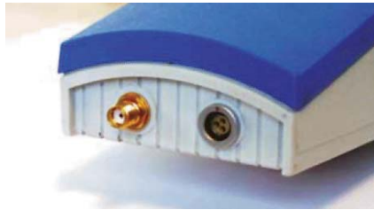
DCF-77 and GSM Antenna Terminal
