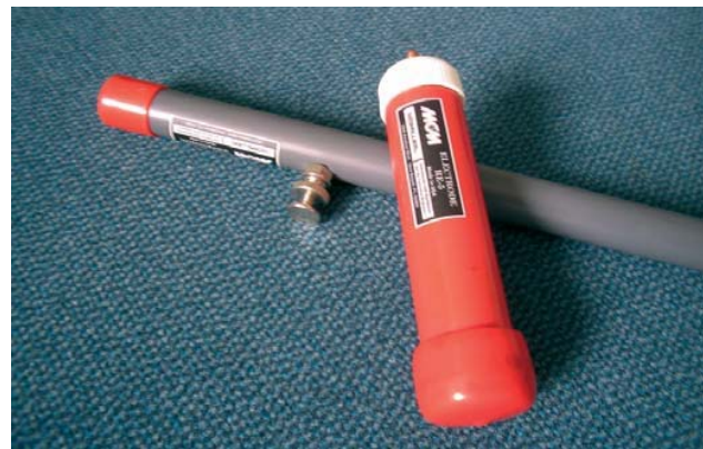
Reference Electrode Cu/CuSO 4 for use in soil and (with submersible adapter) for use in water Model: MILLERRE-5
