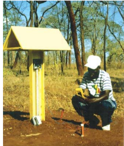
Type - CR - For checking interference effects between the protected pipeline and other pipelines or structures as well as pipeline -to- soil potential measurements
